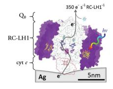
A novel biohybrid photocathode consisting of photosynthetic complexes is revealed on a nanostructured silver electrode. This photocathode nets record photocurrents up to 416 μA cm<sup>-2</sup> in part thanks to a 2.5-fold plasmon-enhanced light harvesting efficiency.
