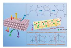
A charged sponge-like membrane with a pore-wall covered imidazolium-based crosslinked structure is designed and fabricated. The prepared membranes exhibit excellent selectivity and stability for vanadium flow battery application.
