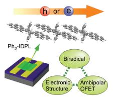
A singlet biradical nature enables high mobility comparable to that of amorphous Si in organic field-effect transistors (OFETs). This paper focuses on the electronic structure and electrical properties of OFETs of a delocalized singlet biradical hydrocarbon, the diphenyl derivative of s-indacenodiphenalene (Ph<sub>2</sub>-IDPL). Ph2-IDPL holds significant promise as a new semiconducting material for high-performance organic devices.
