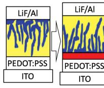
A cross-linkable donor polymer is developed and used as the underlying layer to improve the vertical composition distribution of donor:acceptor in the active layer of polymer solar cells (PSCs). With the improvement, the regular PSC device based on PTB7:PC71BM active layer exhibits power conversion efficiency increase from 7.41% to 8.55%.
