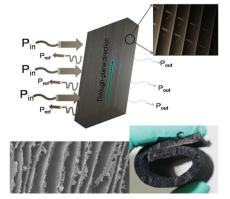
Lightweight, flexible and anisotropic porous composites are assembled by a simple freeze-drying method. The composites contain wide range of mass ratios of multiwalled carbon nanotube in waterborne polyurethane matrix, and show giant electromagnetic interference shielding effectiveness, with the relevant specific shielding effectiveness greater than other shielding materials ever reported.
