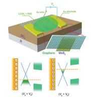
Using monolayer MoS2/graphene heterostructures to construct electric doublelayer devices with an ion-gels dielectric, the possibility of tuning the photoluminescence properties through electrochemical gating is realized. This tunability can be achieved by either modulating the carrier densities of the counterparts or the band alignment at the interface, and the dominant factor determining the PL tuning can be determined.
